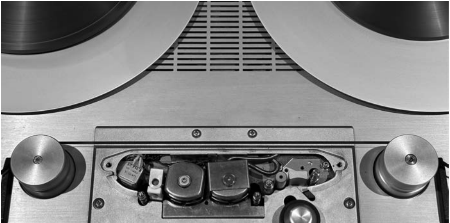
Figure 9. Winding a Pyral CJ87 tape on a Studer A812 with the tape routed behind the head block. The head block cover was removed for more visibility. Source: the author.
