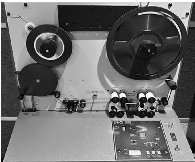
Figure 8. BOW Industries Model 532 cleaning an open reel tape. Source: the author.
