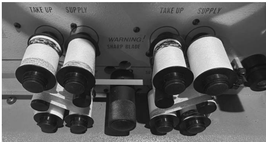
Figure 10. Cleaning tissues from BOW Industries Model 532 showing black traces left by tape shedding on the tape's recorded side. Source: the author.
