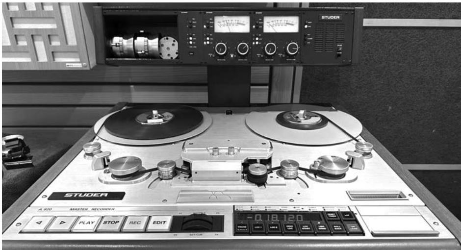
Figure 15. Studer A820 tape reproducer with special azimuth adjustment knobs on the top of the headblock cover. Source: the author.
